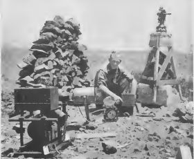
CAMPSTE: On top of Jamanota, Geodesist Hook set up this observation camp. The concrete block on which is mounted the theodolite on its wooden support is the "station." Placed by the government, it is never moved. CAMPAMENTO: Na top di Jamanota, Sr. Hook a traha e campo di observacion aki. E bloki di concreto cu e "theodolite" ariba ta e "station" di traha mapa.
